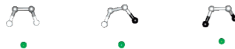
Figure 2. Complexes between Pb(II) and ethyleneglycol (EG), 2-aminoethanol (AE), and ethylenediamine (EDA), optimized at the BLYP/TZVP level combined with CRENBL RECP for the metal. The black color is for N, gray for C, and white for O atoms; the H atoms were suppressed for simplicity.
